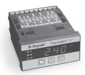
he GPC temperature monitor provides a compact, easy-to-use interface and display for process instruments. This low-cost 1/8 DIN digital panel meter comes standard with features which are optional on other panel meters in this price range. The GPC monitor accepts inputs from any 0–5V sensor, 4–20mA sensor or thermocouple type J, K, E, N, R, S, T. In addition, the monitor can be used with many Raytek noncontact, infrared temperature sensors.
